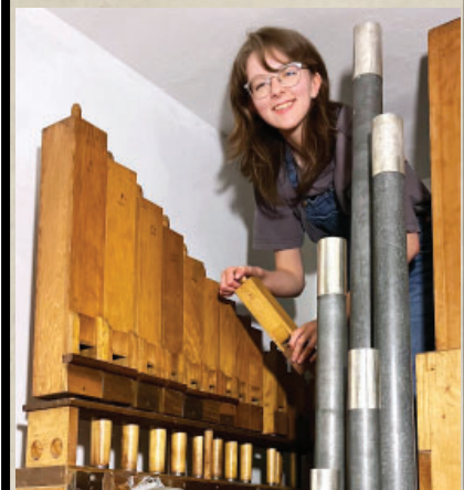
Calling in the pros: Sean Reed, 32° and his daughter Reiley (above) keep the 1926 Kilgen & Sons organ in great working order. Here, Reiley is adjusting a tuning stopper in a wooden flute pipe, which was stuck.
